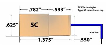
The 5C base is an excellent end cap combining proper lamp support and electrical isolation. Often times it can be substituted for the 4C end cap. The 5C is used on American M&M, Amjo, Brewer UV, Cefla, Gallus, Ko-Pack, Liberty Apollo, Svecia and VTI lamps.
