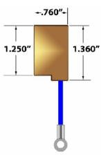
Another side wire base whose main attribute is small size. We call this GEW end cap as it is found exclusively on GEW–style label curing equipment. Due to ceramic size, take care when installing lamps with 1.360" GEW base. They are easily snapped.
