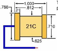
The 21C end cap is used in credit card and label printers. It provides excellent support and dielectric strength.
