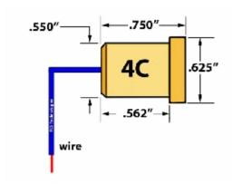
The 4C end cap is typically used on screen printing lamps. Its main attraction is its small size. There are better choices in end caps (see 5C) as its lack of physical support and poor insulating value can contribute to lamp problems. The 4C end cap is used on Dorn SPE, FMA and M&R style lamps.
