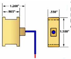
The HOK end cap is used on lamps found in Argon Equipment. We call it HOK end cap as it is used in Philips HOK series UV curing lamps. Take care when installing lamps with this base as one can easily snap the lamp end.
