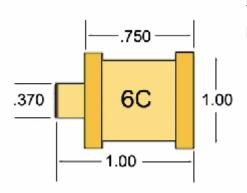
The 6C base is primarily used on Aetek style label printing lamps. It provides excellent support.
