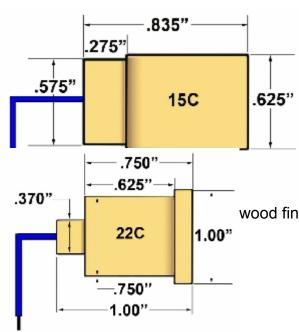
The 15C end cap has a nice overall design where space is at a premium and still maintains structural integrity.
