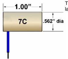
The 7C ceramic end cap is used on several Eye Graphics lamps
