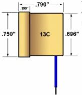
The 13C end cap is often used on optical media (CD DVD) lamps where compact size is paramount. Wire comes out the rear side to minimize lamp installation length.
