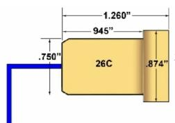
Primarily used on lamps of German manufacture, the 26C provides excellent support and electrical isolation. Its main drawback is its weight. Take care when
