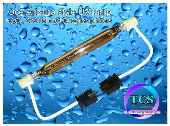
Oce—Cannon Arizona printers use two (2) lamps, one on each side of the carriage. To reduce gloss banding and maintain equal UV dosage, replace both UV lamps at the same time. Additionally, we recommend replacing lamp housing air filters during bulb change procedure.
