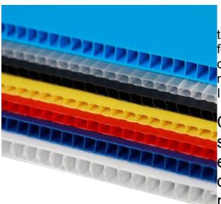
Corrugated plastic is a light weight, tough material which can be easily cut and formed. It is offered in a wide range of colors and thicknesses. It is known under many trade names including Coroplast, IntePro, Correx, Corflute and others.
